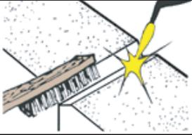
Brush surface to be repaired thoroughly under heat to break up surface oxide.
