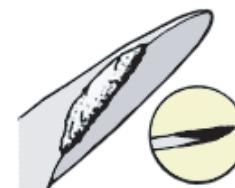
Turn and tin bevelled side, building out the blade slightly larger than its original size. Grind damaged edges to a 45 bevel. Pitch propeller to standards.
