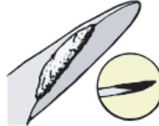
Turn and tin bevelled side, building out the blade slightly large than its original size. Grind damaged edges to a 45 bevel. Pitch propeller to standards.
